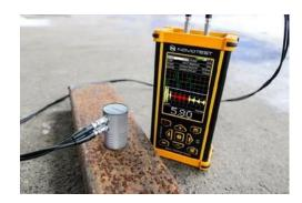
The electromagnetic-acoustic thickness gauge allows user to measure the thickness of metal products with one-side access without using couplant through a substantial gap (up to 6 mm). This significantly reduces the material- and laboriousness of the measurement process.
