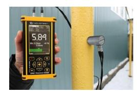
EMA technology generates waves directly in the material (ferromagnetic and paramagnetic), thus allowing measurements to be carried out under the coating, with a poorly prepared surface or even air gap, which may not be feasible with traditional methods.
